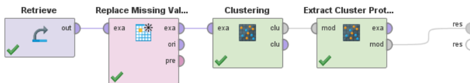
Obr. 12.18 Proces extrahovania prototypov operátorom Extract Cluster Prototypes
